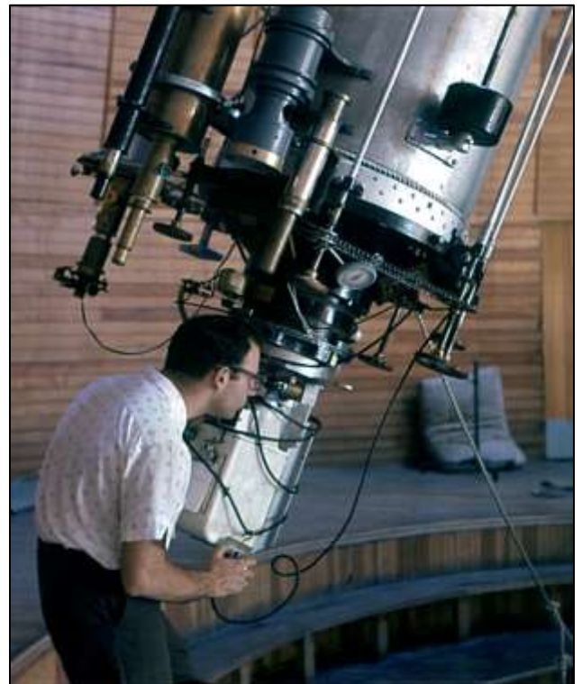
Figure 11. Howard Cohen at the Clark with attached 70 mm Hulcher camera. Image: © 2011 H.L. Cohen
