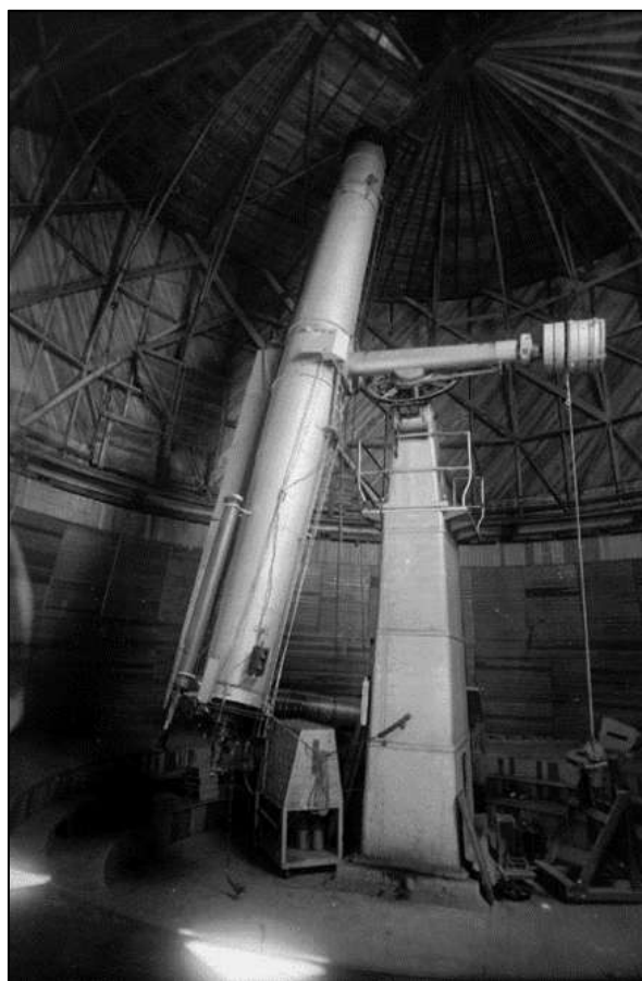
Figure 1. The Lowell Observatory 24-inch Clark refractor used to map the Moon for Project Apollo . Note 6-inch finder and 12-inch guide scopes. Lowell Photo Archive.
